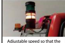
Adjustable speed so that the red light is on in order to inform speed excess
